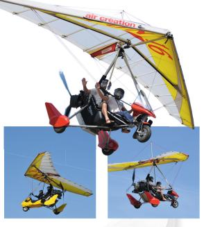
Kevlar reinforcements, UV-protected Trilam fabric, minimum weight (45 kg [99 lbs]) but maximum resistance (+6 /-3g to 462 kg [1,018 lbs]), all are standard for overwhelming safety and durability.
